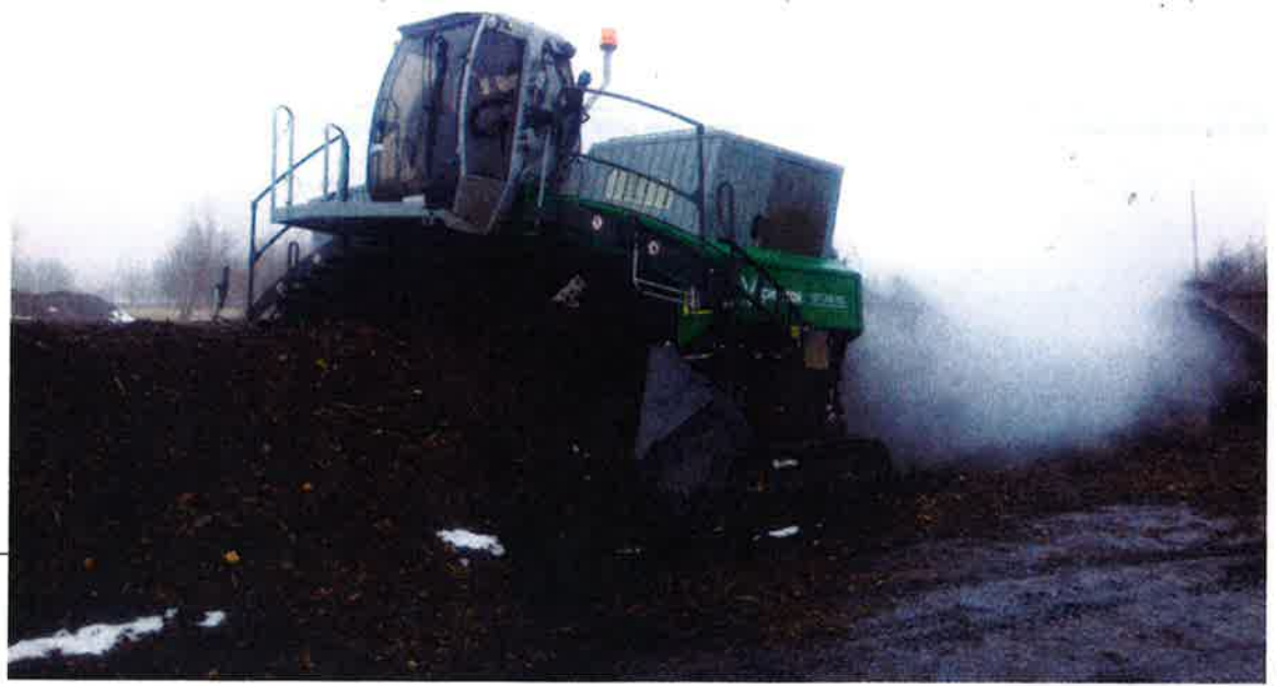
Track type straddle turner turning in very wet conditions.
