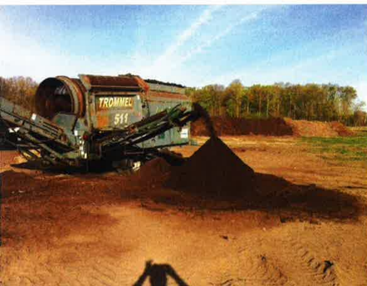
Left: Finished compost screening in preparation for sale at the Ashley operation. Right: Routine grinding operations at the DeKalb County compost facility. Images courtesy of the Northeast Indiana Solid Waste District.
